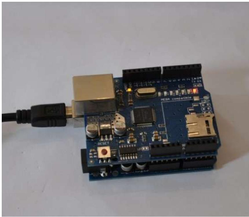
arduino w5100 test code:
