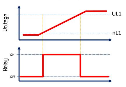
The relay is on when the input voltage is outside the UL1, nL1 range. Off when it is inside.
