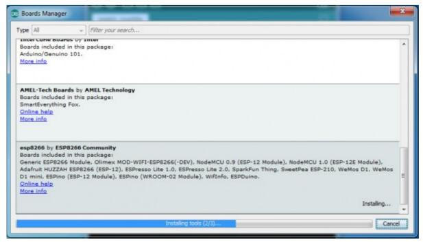
After installation, close the window and go to Tools> Board and see the list of available devices on the chip programming ESP8266
