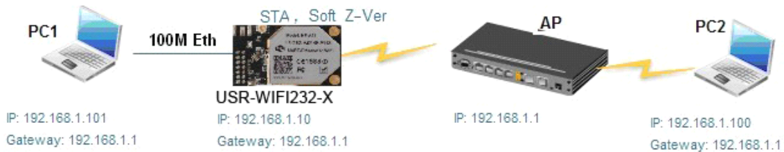
Figure 21 USR-WIFI232-X Ethernet Interface Networking (As STA, Z-Ver)
