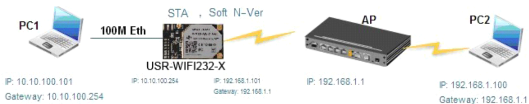
Figure 20 USR-WIFI232-X Ethernet Interface Networking (As STA, N-Ver)
