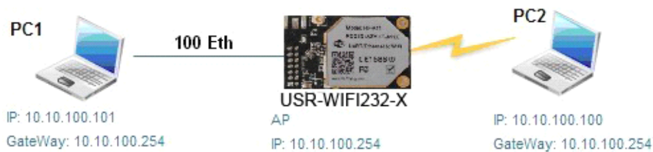
Figure 19 USR-WIFI232-X Ethernet Interface Networking (As AP)
