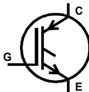
Depletion mode IGBTs are characterised by the fact that current can flow between the collector and emitter when there is zero voltage across the gate-emitter terminals.
