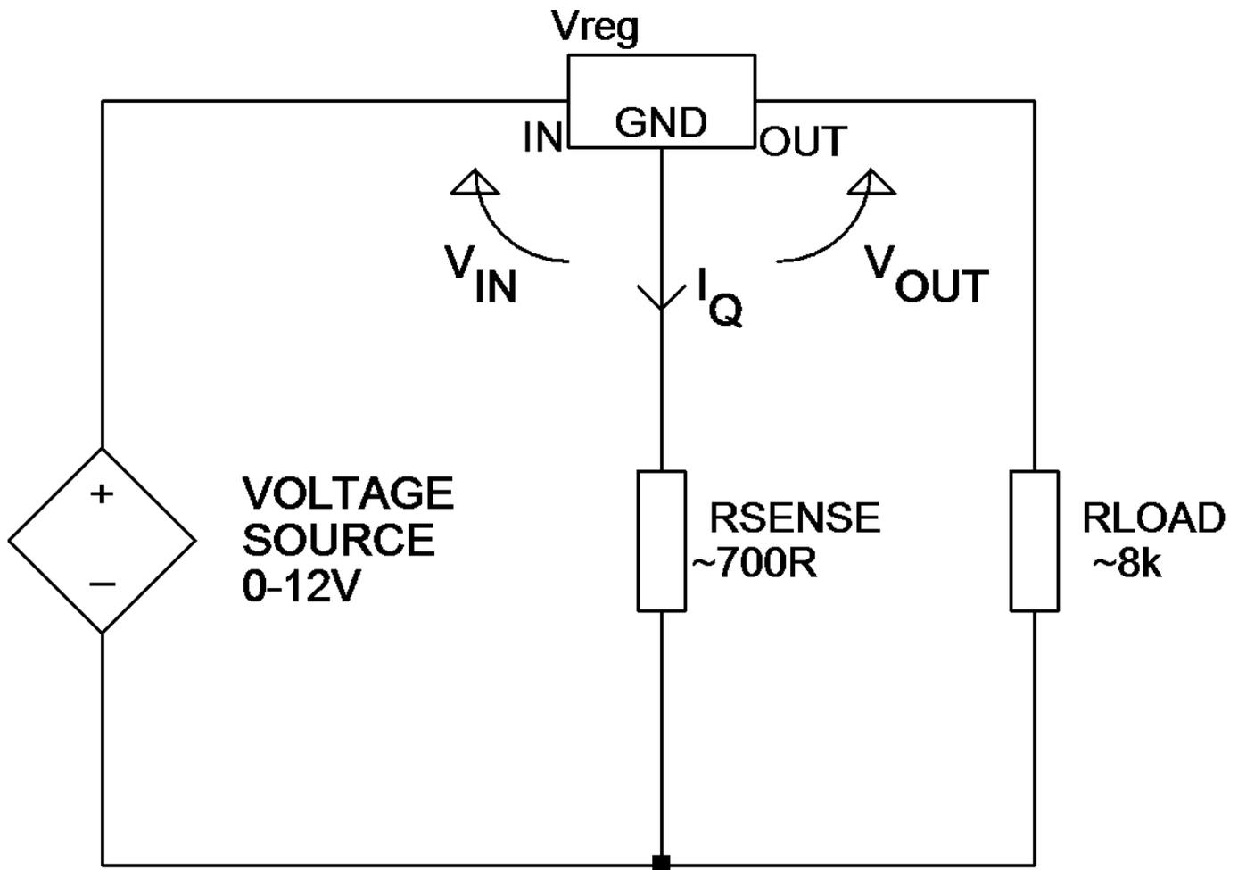
The test circuit shown here is used for the analysis of voltage regulators (positive regulators in this example). Note that the range of regulator voltages supported will depend on the quiescent current ( $I_Q$ ). A higher quiescent current will cause more voltage to be dropped across the sense resistor and yield less voltage for the regulator itself.
