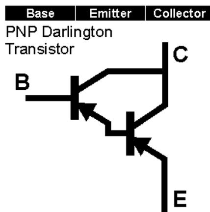
Note that the component schematic is displayed in colour to illustrate which colour test lead is connected to each component lead.
