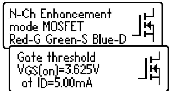
Pressing **scroll-off** will then result in the gate threshold of the MOSFET being displayed.
