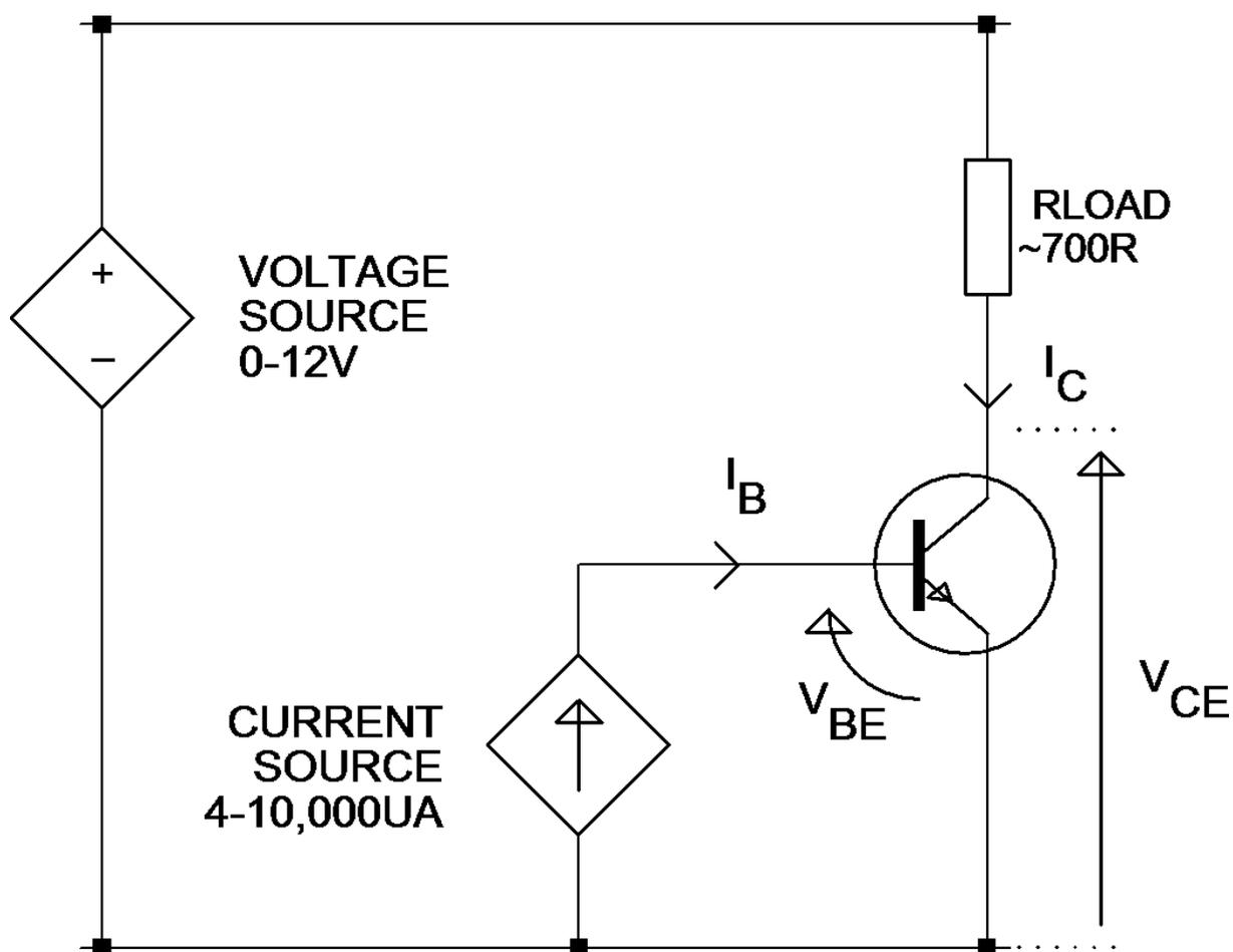
Example shown is for an NPN transistor. Polarities are reversed for PNP devices.
