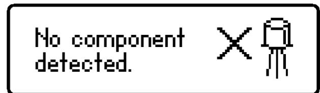
If the component is not a supported component type, a faulty component or a component that is being tested in-circuit, the analysis may result in the following message being displayed:
