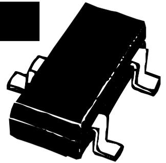
The *DCA Pro* will identify multiple diode junctions between the probes. For three terminal devices such as SOT-23 diode networks, all three test clips must be connected.
