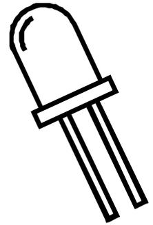
Bicolour LEDs are generally available in two main varieties; 2-lead and 3-lead types.
