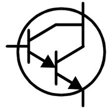
If the device is a Darlington transistor (two BJTs connected together), the unit will display a similar message to this:
