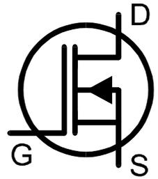
The fairly rare Depletion Mode MOSFET is very similar to the conventional Junction FET (JFET) except that the gate terminal is insulated from the other two terminals. The input resistance of these devices can typically be greater than 1000MΩ for negative and positive gate-source voltages.
