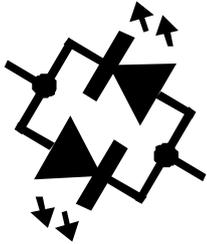
This section describes the testing of 2-lead bicolour LEDs. These types are internally connected in inverse parallel (back-to-back).
