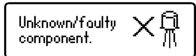
Some components may be faulty due to a shorted junction between a pair of the probes. If this is the case, the following message (or similar) will be displayed:
