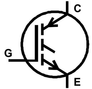
IGBT is an acronym for Insulated Gate Bipolar Transistor.
