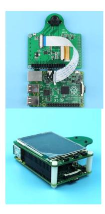
Connect the RaspCAM and Raspberry Pi B+ board Connect the 40pin connector on the RaspCAM board to the pin header on the Raspberry Pi B+ board. Using the plastic standoff spacer between two boards, then fasten the screws.
