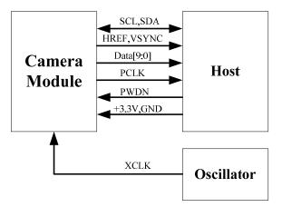
The host may have integrate camera interface like STM32F2 or STM32F4 series MCUs, or ARM9/11 which has dedicate camera port, and DPS like TI TMS320DM series, as well as FPGAs that user can design special logic for camera application. The typical connection between these system and camera module would show like following diagram.
